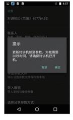
Click the "write frequency for interphone" button, and write all parameters set by APP into the interphone chip once: You can then switch channels by rotating the channel knob. (note: after each modification of the parameters of the walkie-talkie, no matter the analog or digital parameters are modified, the operation of "walkie-talkie write frequency" must be performed before the modified parameters take effect )
